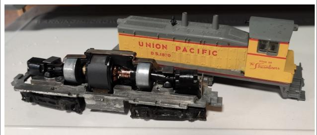
An Athearn SW-7 I bought on eBay. It was in bad condition. It appeared to have been lying in some kind of brown liquid that corroded the die cast chassis. One motor brush was stuck and was not touching the armature. The electrical pieces were rusted and corroded.
