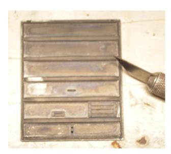
Paint in the corners of the doors and on the board was scratched out with the knife. Body is now ready for painting.
