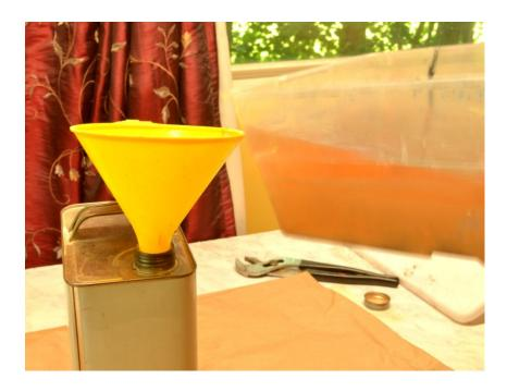
Put the funnel in the can and slowly pour in the alcohol. Some of the alcohol might have suspended paint in it. When you are down to the real dirty stuff, stop. A metal one gallon can is the best solution for storage as the spout has a small opening with a metal cap that seals it. Do not use a coffee can with a plastic lid as this will not seal the container.
