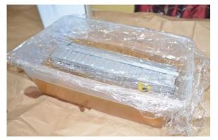
Fill the chamber up half way. With the sample shown, this was around three quarts. I used alcohol that I used previously, that's why it has a red tint. Cover the chamber with plastic wrap. The fumes will work on the area of the body not submerged.
