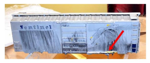
The red arrow shows the yellow and blue lettering melted at the bottom of the body.
