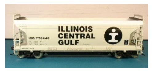
Lettering may be ink and not paint and therefore will be difficult to remove. During most of the stripping I have done, the white lettering is the last area to melt off. It traps the paint colors of the body underneath it. I tried to strip an Atlas HO 2-bay covered hopper and all the paint came off except for the black lettering "Illinois Central Gulf." I had to paint over it.
